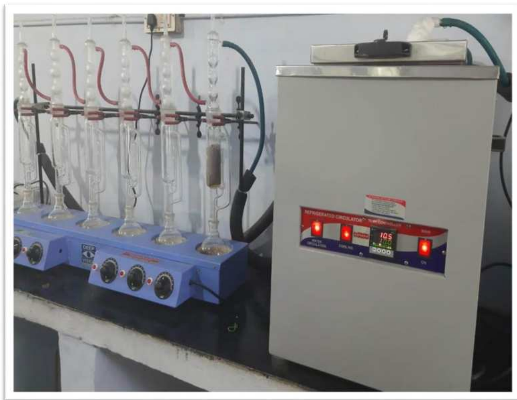
Fig 3.4 Brassica Oleracea var.botrytis EXTRACTION USING SOXHLET EXTRACTOR
