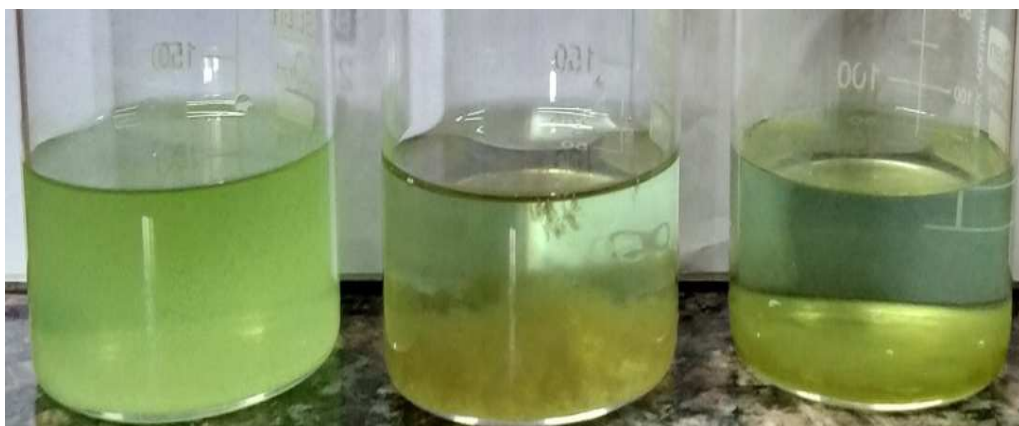
Plate 11: Copper oxide nanoparticles synthesis by treating 1m of aqueous copper sulphate solution with 10 mg of Lucas aspera stem extract (Water ethanol, chloroform)
