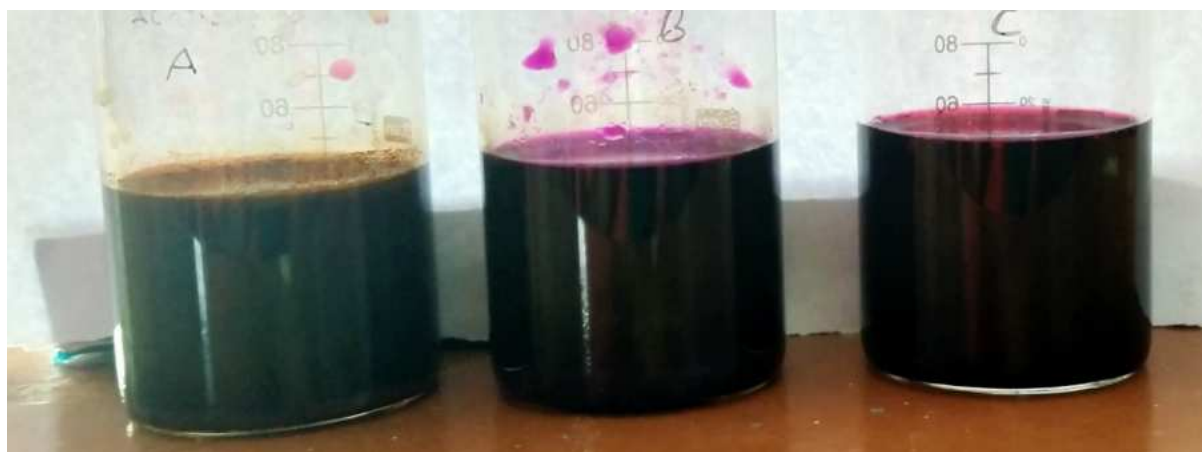
Plate 24: Manganese oxide nanoparticles synthesis by treating 0.2 m of aqueous potassium permanganate solution with 10 mg of Pedaliium murex leaf extract (Water ethanol, chloroform).
