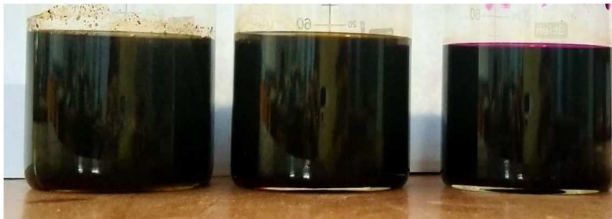
Plate 21: Manganese oxide nanoparticles synthesis by treating 0.2 m of aqueous potassium permanganate solution with 10 mg of Acalypha indica leaf extract (Water, ethanol, chloroform)
