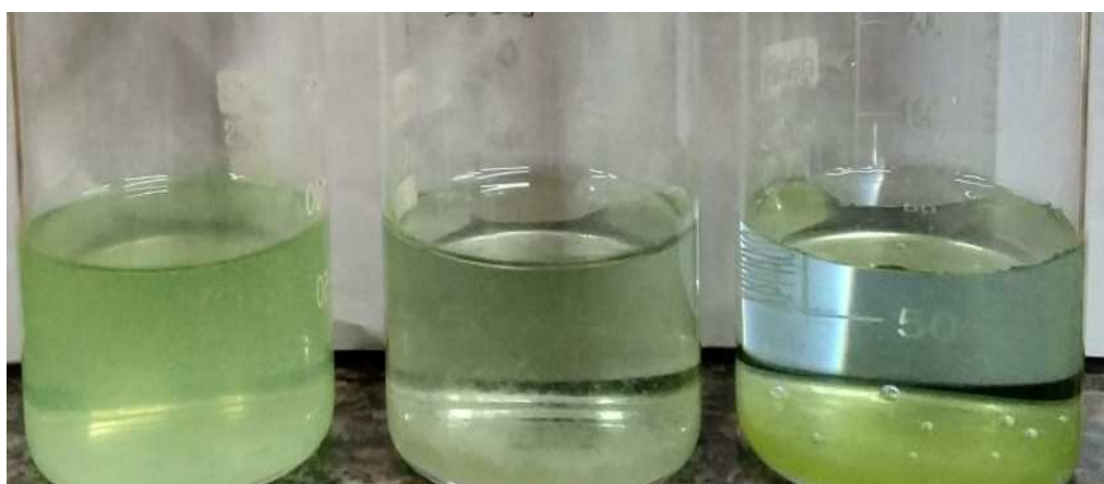
Plate 12: Copper oxide nanoparticles synthesis by treating 1m of aqueous copper sulphate solution with 10 mg of Pedaliium murex stem extract (Water ethanol, chloroform).
