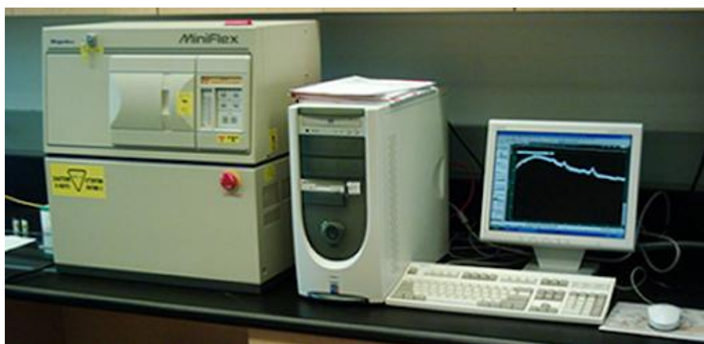
Fig : 4.6.1 schematic representation of XRD spectrometer
