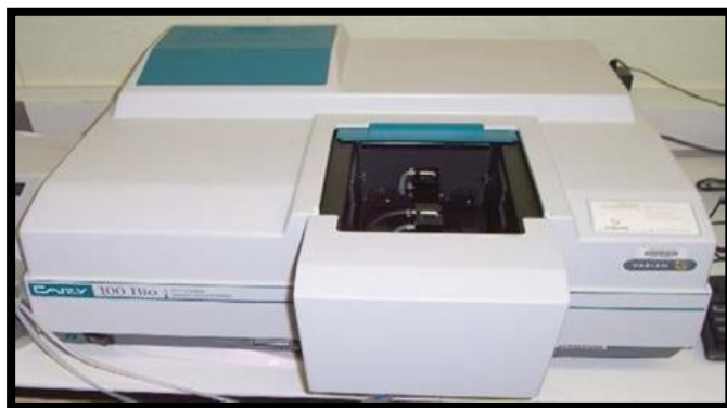
Fig : 4.3.1.1 schematic representation of UV – Visible spectrometer
