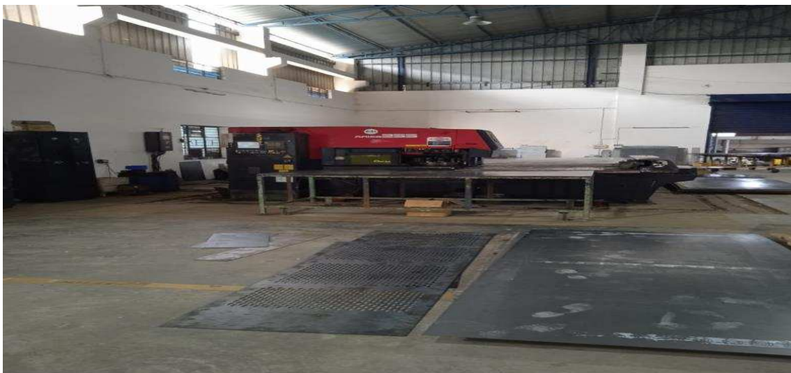
Fig. 3.3.3 Punching machine with punched sheets
