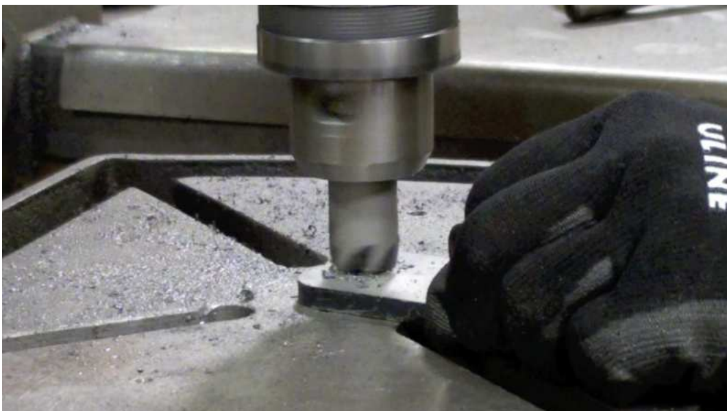
Pictorial Representation of Counter Sinking Operation (Fig 6.10.2)
