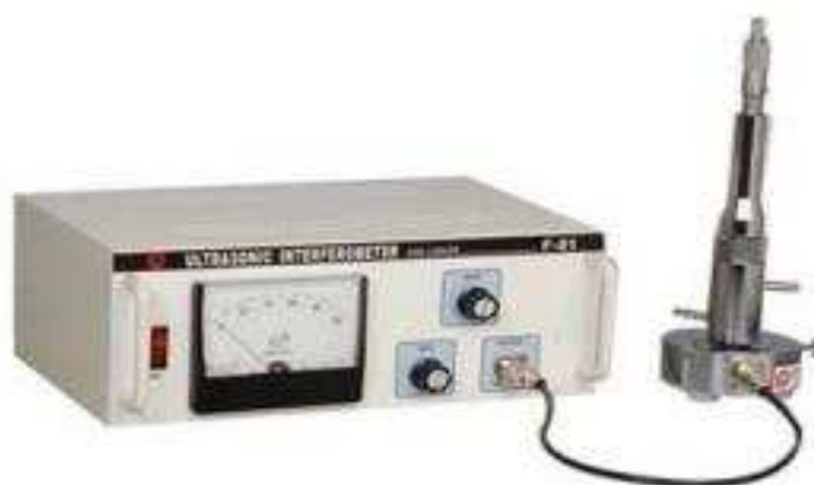
Fig3.1: Experimental setup for ultrasonic interferometer.
