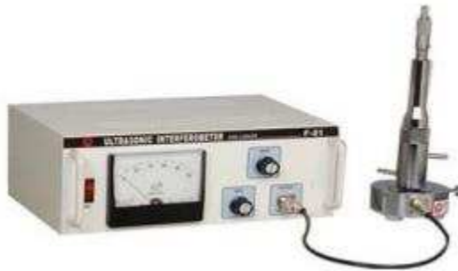
Fig 1: Experimental setup for ultrasonic interferometer.
