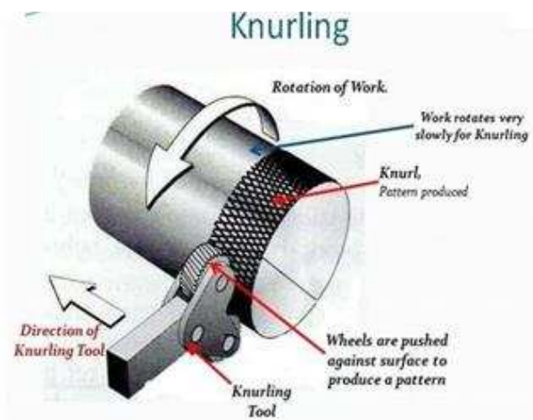
Pictorial representation of Knurling Operation (Fig 6.8)
