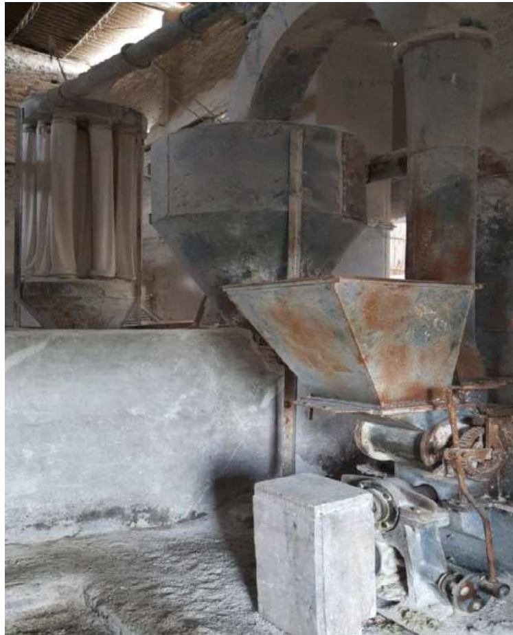
Fig.7.1 Picture consisting of a pulverizer, filter and an elevator.
