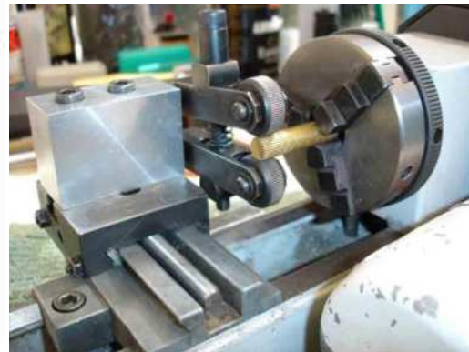
Pictorial representation of Knurling Operation (Fig 6.8)
