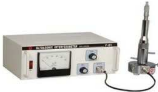
Fig 3.1: Experimental setup for ultrasonic interferometer
