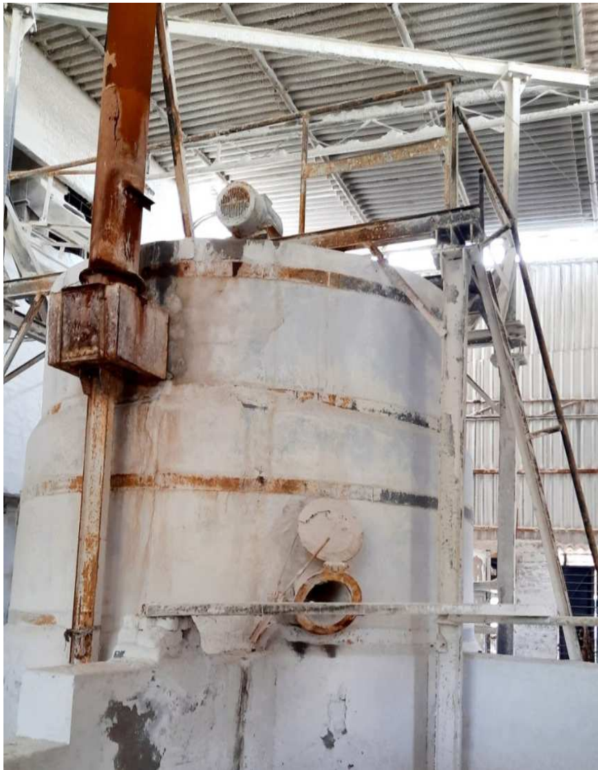
Fig.7.3 Picture of boiler containing an opening for firewood input.
