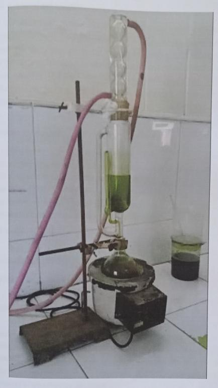
Fig 3: Extraction Of Sample Using Soxhlet Apparatus
