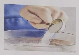
Fig: 25 Chitosan mixed with citric acid
