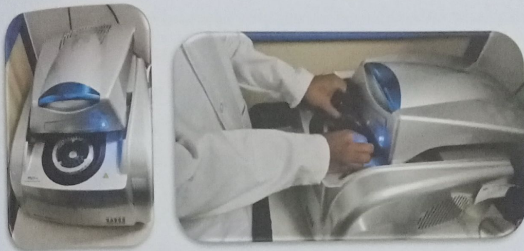
Figure 5: mRNA Expression Analysis using Qiagen Rotor Gene qRT PCR Instrument
