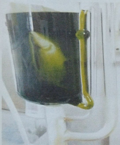
Figure 3.2 Soxhlet extraction of the extract
