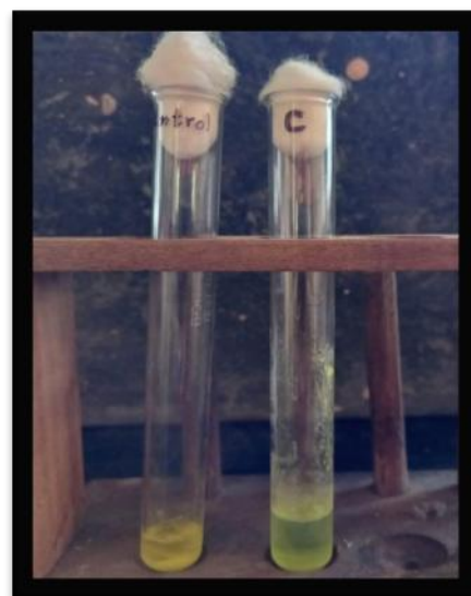
Figure 3: Synthesized Calcium Nanoparticles using the Shell Extract of Harpulina lapponica
